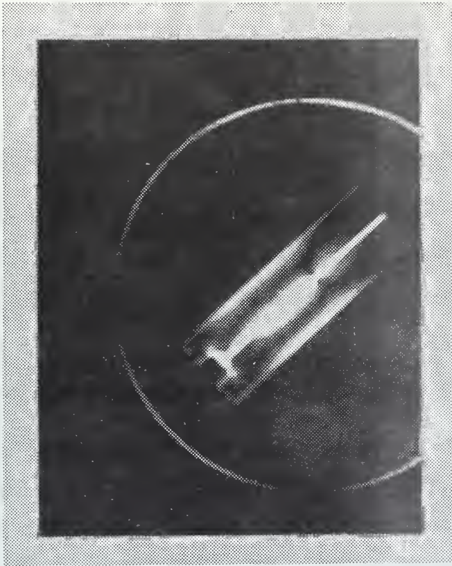
Figure 9. Stresses shown are caused by \text{KNO}_3 salt which has solidified in the crack. The specimen had been immersed in the \text{KNO}_3 bath at 365^\circ\text{C} for thirty minutes.
