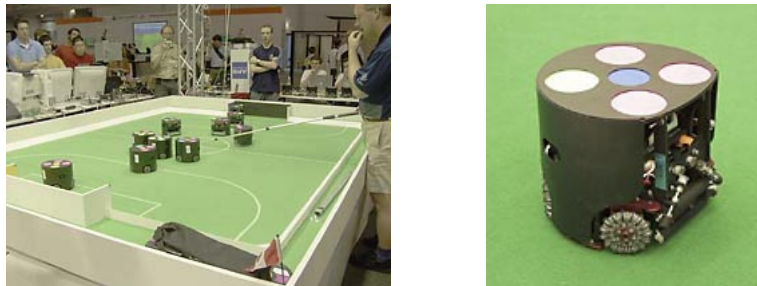
Figure 9. Robo-soccer platforms built by Cornell University in 2003 ( www.cornell.edu )
