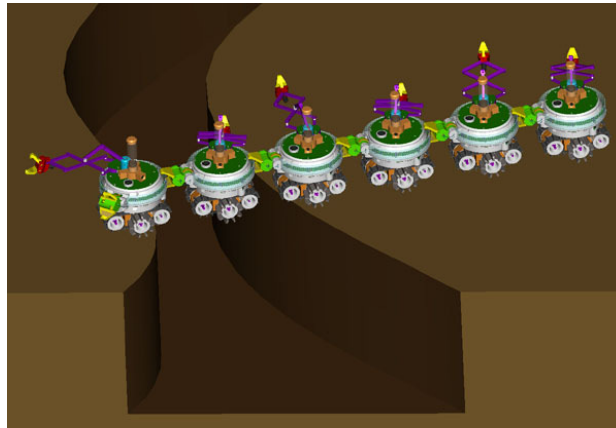
Figure 11. Swarm-bot project simulation of concept of crossing gaps (Dorigo, 2004)
