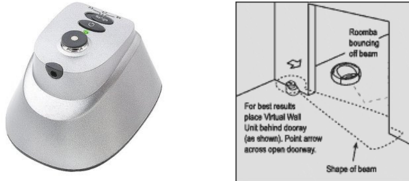
Figure 24. iRobot Virtual Wall Unit ( www.irobot.com )
