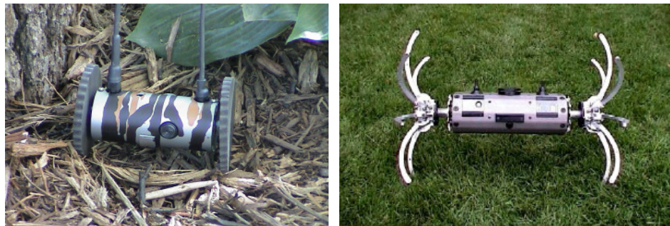
Figure 7. Left: A recent ThrowBot variant called the COTS-Scout. Right. A larger ThrowBot variant, the “MegaScout” with actuated-wheels (Kratochvil, 2003)
