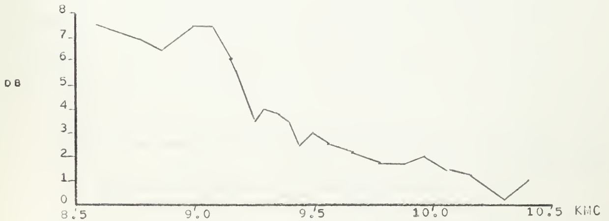
REFLECTED POWER AT TE 20 SINGLE MODE PORT IN DB BELOW INCIDENT POWER VS. FREQUENCY.
