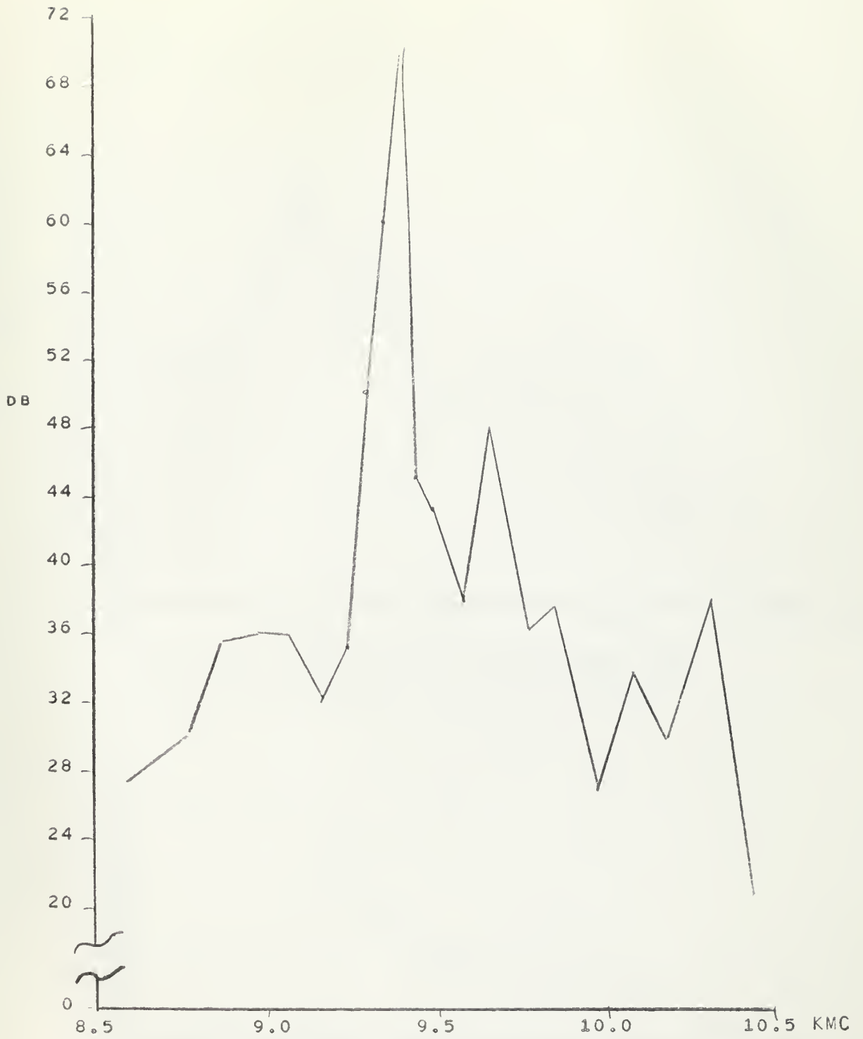
ISOLATION BETWEEN TE_{10} AND TE_{20} SINGLE MODE WAVEGUIDE PORTS VS. FREQUENCY
