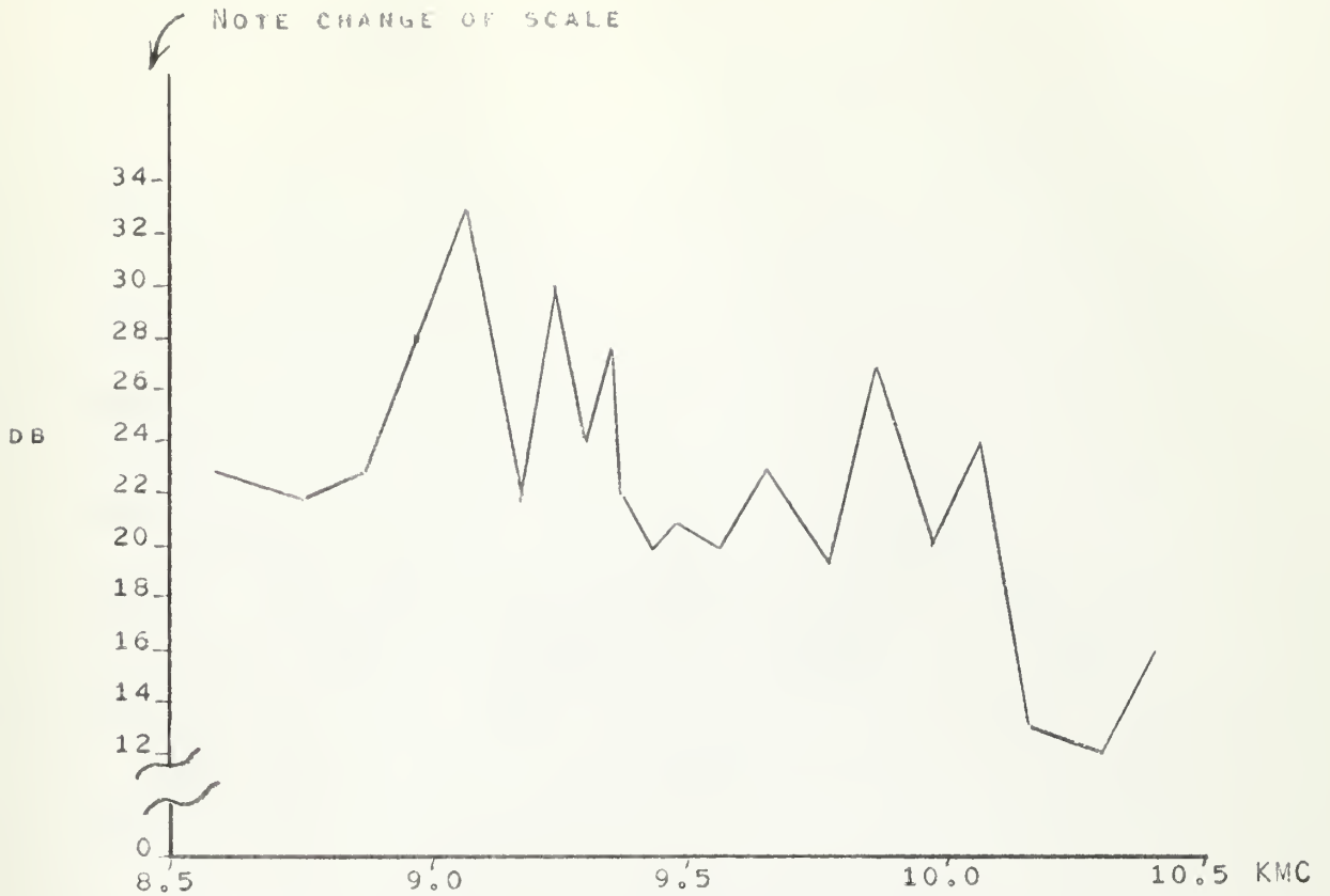
REFLECTED POWER AT TE 10 SINGLE MODE PORT IN DB BELOW INCIDENT POWER VS. FREQUENCY
