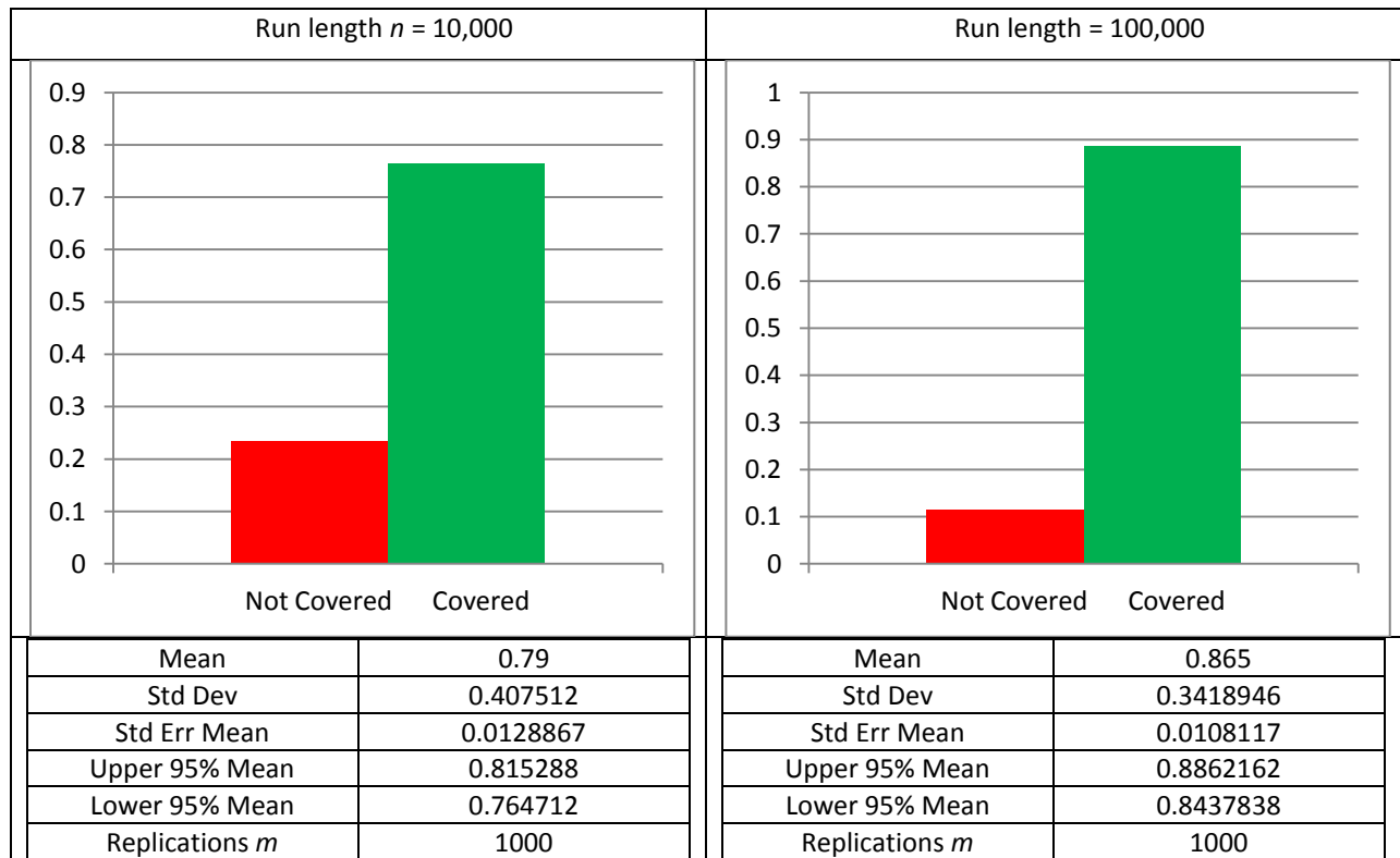
Figure 1: Statistics of the indicator variable recording coverage of the 90% confidence interval on the mean delay in queue for a simulated M/M/1 queue.
