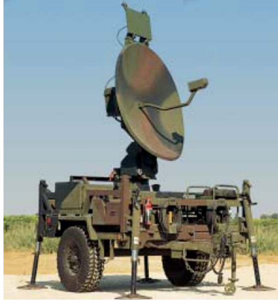
Figure 14. A Ground Data Terminal – EL/K-1861 [From 17].
