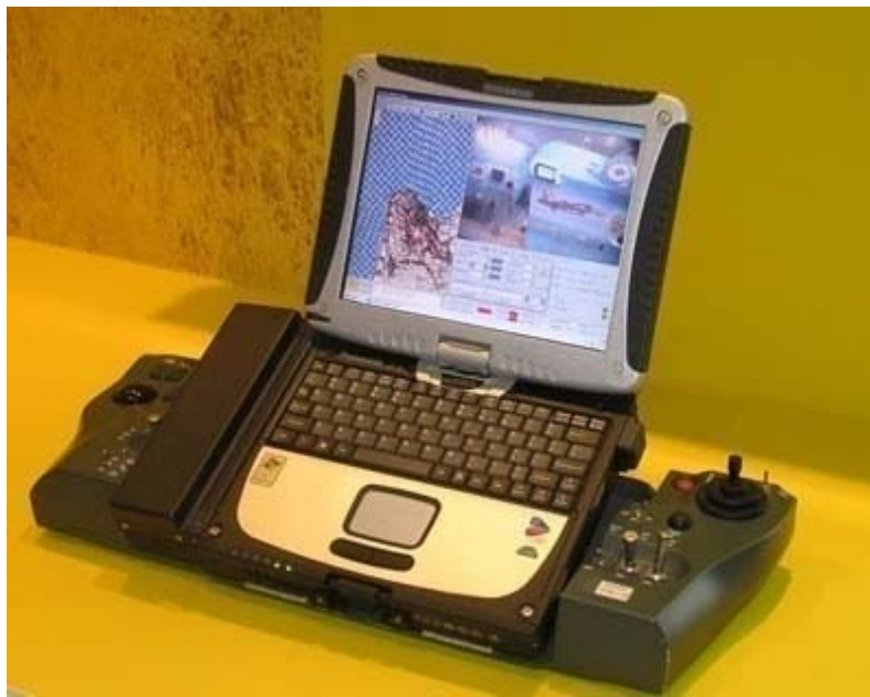
Figure 10. A Handheld Computer Serving as the Ground Control Station for the Skylark Mini UAV [From 16].
