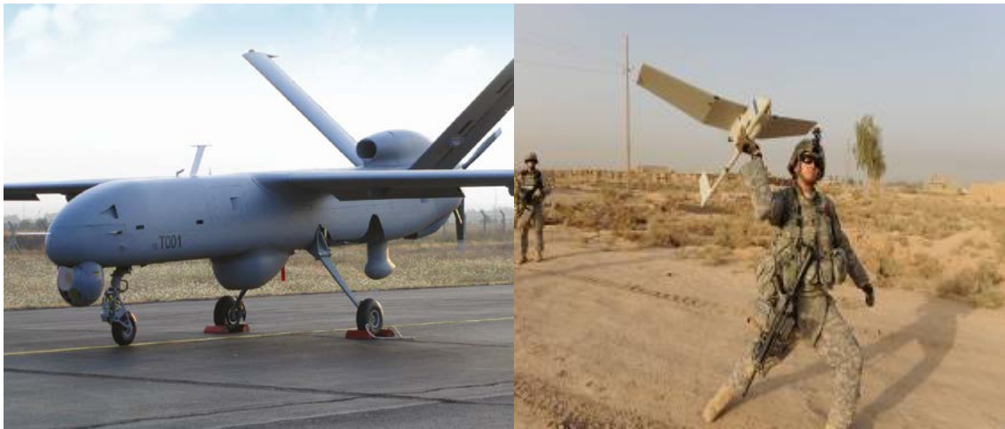
Figure 5. ANKA type of UAV (left) and a hand-launching type of Raven (right) (from UAVGLOBAL, 2014; Unmanned Ground, Aerial, Sea and Space Systems, 2011).
