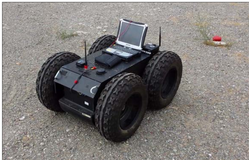
Figure 29. RMP-400 Equipped with ARAM Sensor
