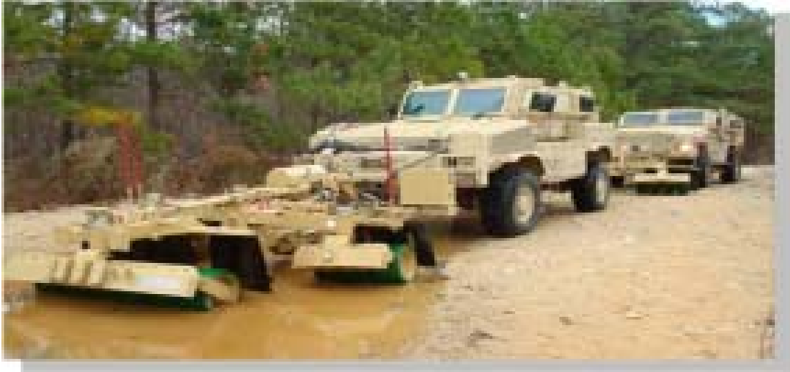
Figure 9. Full-width RG-31 with Track-width Rollers (OIF) Installed (PM IEDD/PF Product Office, 2009, p. 0002-7)
