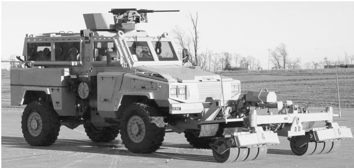
Figure 8. RG-31 with Track-width Rollers (OIF) Installed (PM IEDD/PF Product Office, 2009, p. 0002-16)
