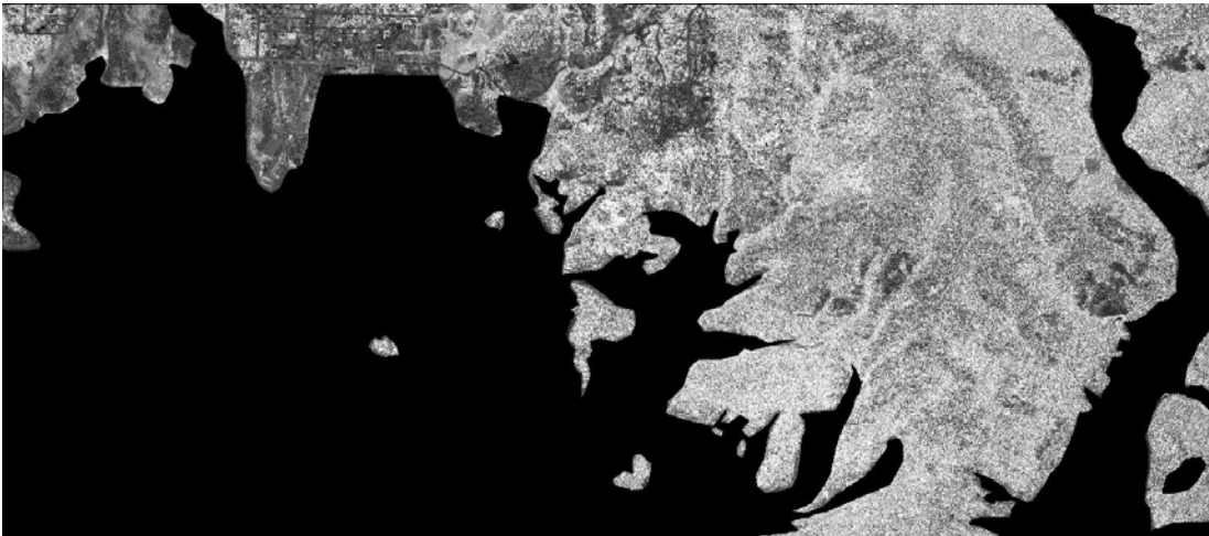
Figure 26. MTMF ratio image of green healthy trees from September 2006 QuickBird data created by comparing image pixel spectra to regions of interest. Image size is 5.952 km by 2.62 km.
