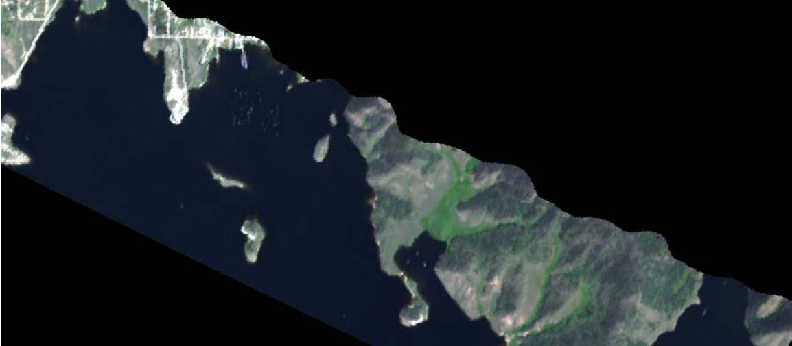
Figure 15. Spatially adjusted, atmospherically and empirically corrected, and registered AVIRIS image of study area from 2011. Image size is 5.952 km by 2.62 km.
