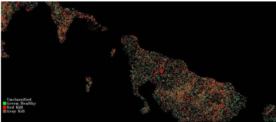
Figure 35. MTMF ratio classification map created by matching library spectra to image pixel spectra from August 2011 AVIRIS data. Image size is 5.952 km by 2.62 km
