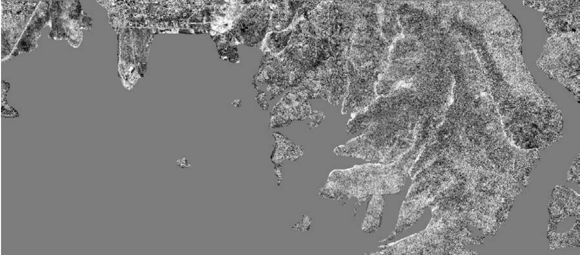
Figure 19. MF score of young green lodgepole pine trees from September 2006 QuickBird data created by comparing image pixels to library spectra. Image size is 5.952 km by 2.62 km.
