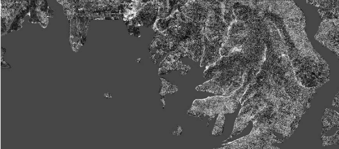
Figure 25. MTMF ratio image of young green lodgepole pine trees from September 2006 QuickBird data created by comparing library spectra to image pixels. Image size is 5.952 km by 2.62 km.
