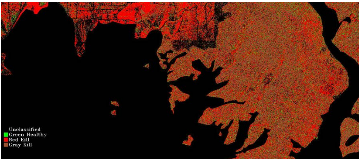
Figure 34. MTMF ratio classification map from June 2011 IKONOS data created by matching spectral library plots to image pixel spectra. Image size is 5.952 km by 2.62 km
