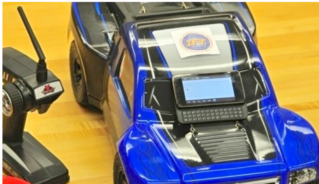
Figure 7: A Nokia N900 phone is attached to each car
