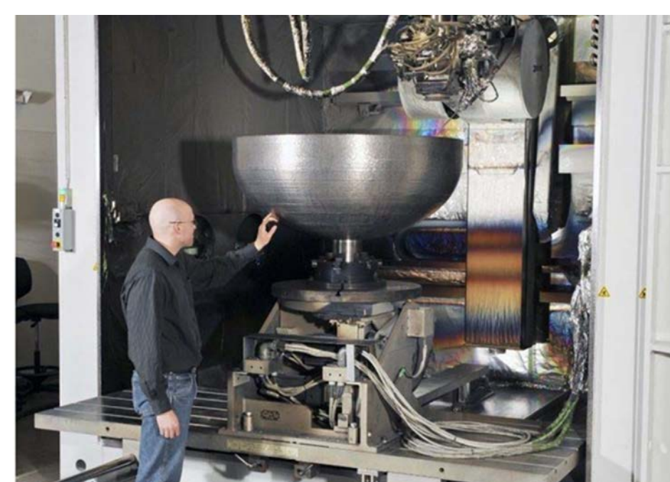
The EBAM metal 3D printer at Lockheed Martin's manufacturing facility located in Littleton, CO. Source: Grunewald (2016).
