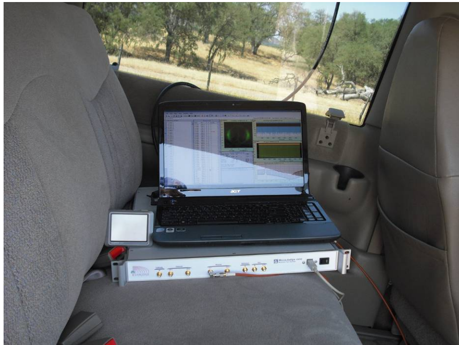
Figure 22. Collection Suite (GPS, Laptop, and WaveJudge).
