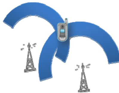
Figure 2. Illustration of Overlapping Timing Advance Range Rings.
