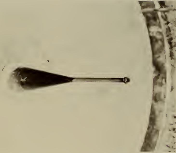
Fig. 6. A close-up view of the probe and turbulence screen. The disc from which the cavity is formed can also be seen.
