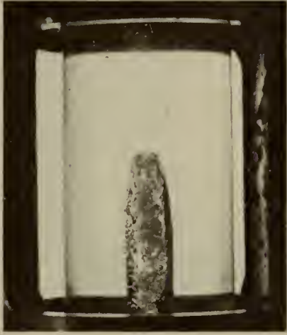
Fig. 15. Water cavity. T=109.5^{\circ}\text{C} , v=19.44 ft/sec, l=1\frac{3}{8} in.
