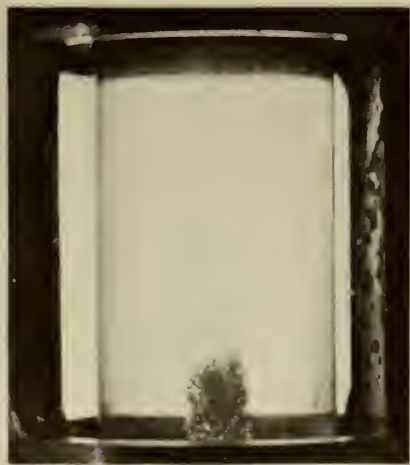
Fig. 8. Water cavity. T=98.1^{\circ}\text{C} , v=18.42 ft/sec, l=13/16 in.
