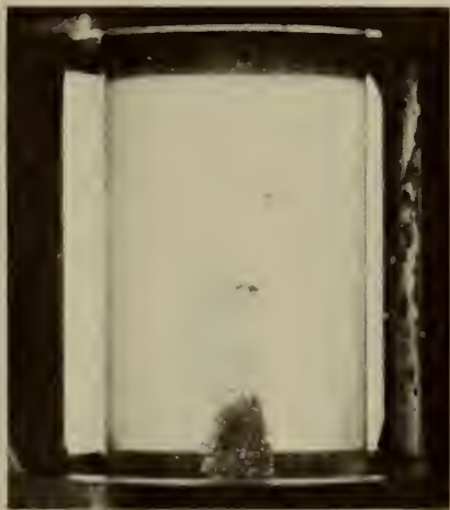
Fig. 9. Water cavity. T=105.6^{\circ}\text{C} , v=18.84 ft/sec, l=13/16 in.
