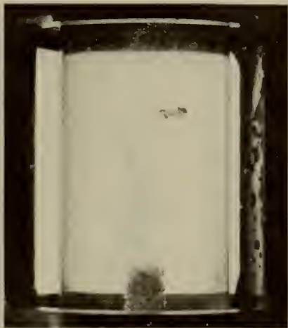
Fig. 10. Water cavity. T=109.9^{\circ}\text{C} , v=19.75 ft/sec, l=13/16 in.
