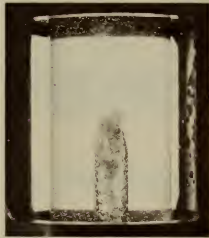
Fig. 16. Water cavity. T=114.5^{\circ}\text{C} , v=18.99 ft/sec, l=1\frac{3}{8} in.
