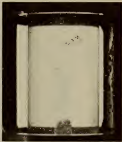
Fig. 11. Water cavity. T=114.7^{\circ}\text{C} , v=19.17 ft/sec, l=13/16 in.
