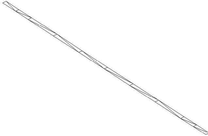
Figure 1: Example of a strip dipole meshed for the method of moments solution.
