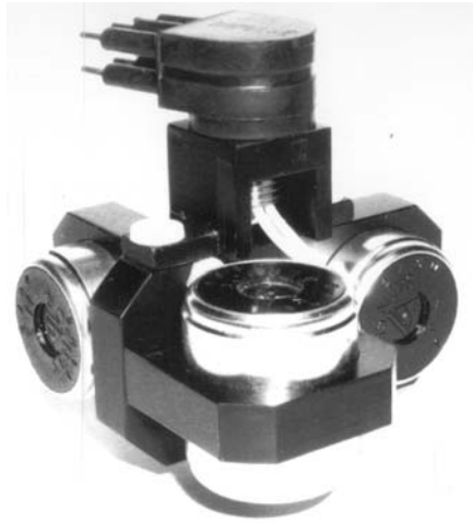
Figure 12. SM-11 geophones mounted on three axes
