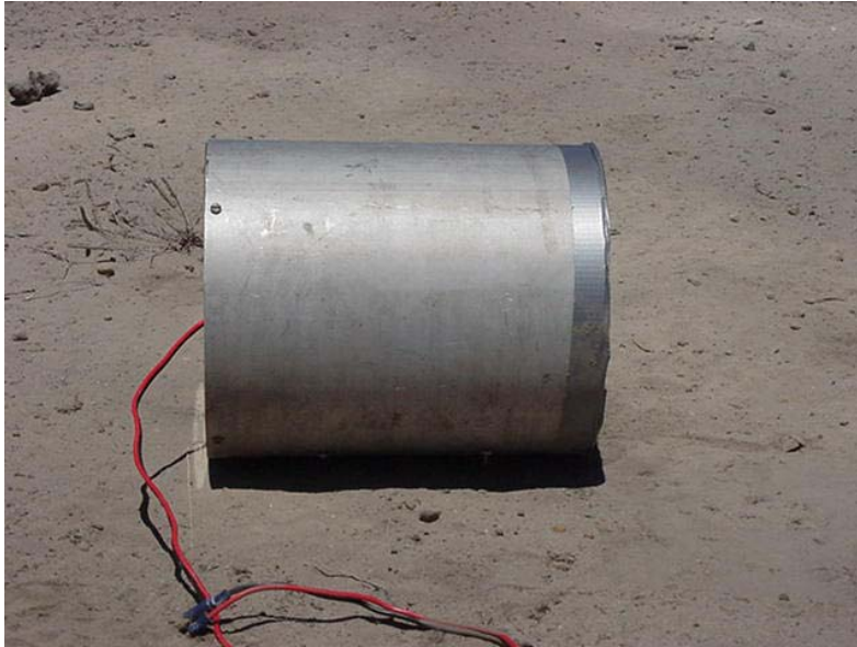
Figure 2. Rolling Line Source Element
