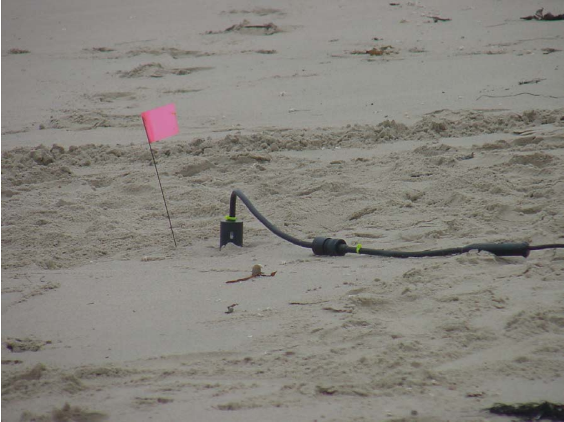
Figure 20. Photo of buried seismometer at 12.2 m (40ft)
