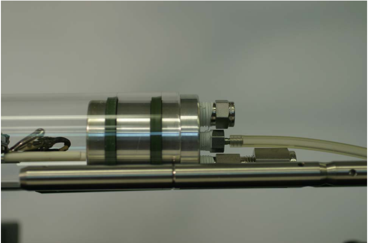
Figure 23: Rear end cap with two gas flow lines and one pressure relief check valve and sectioned aluminum guide rails
