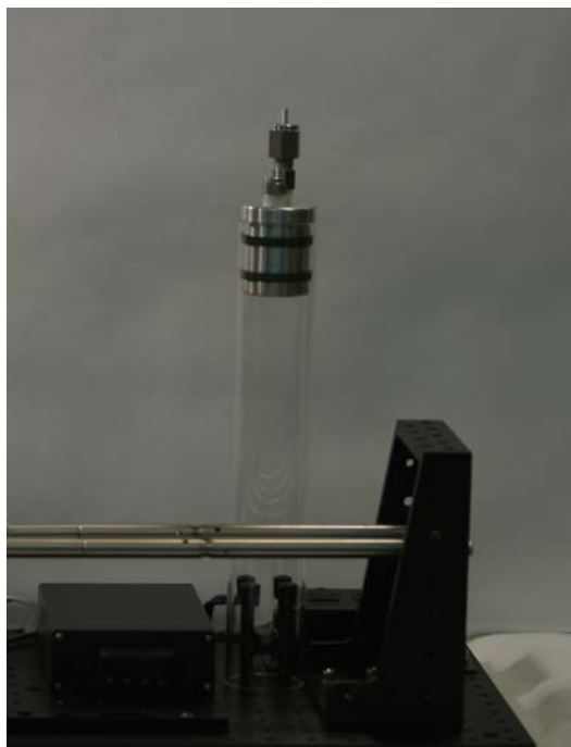
Figure 25: Quartz tube in the resting vertical position on the vertical tube holder
