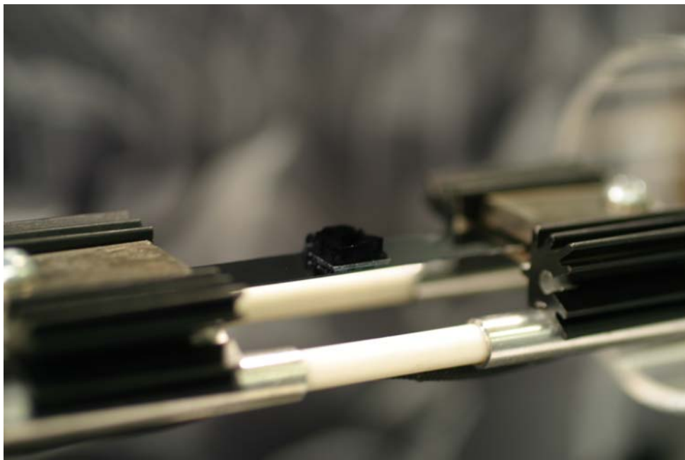
Figure 51: CNT growth in the SabreTube
