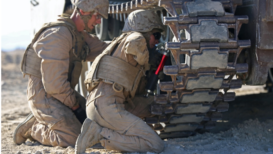
Figure 11. AAV Marines Performing MetID: AAV003: Break and Reassemble Track
