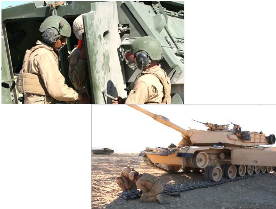
GCEITF Marines replacing an armored hatch panel on an LAV (top left) and repairing an M1A1 track section (bottom right). Source: https://www.dvidshub.net/unit/MCGCE-ITF
