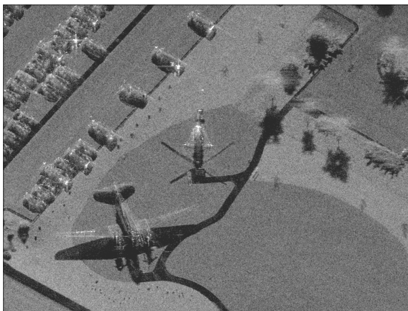
Figure 8. A 4 inch resolution image from Sandia National Laboratories. Note the shadows of the historical airplane, helicopter and trees. (Courtesy Sandia National Laboratories)
