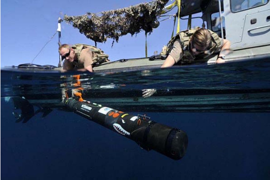
Figure 1. Sailors deploying the MK 18 Mod 2 Swordfish UUV in FIFTH FLEET during IMCMEX 2014 (from Midnight, 2014).
