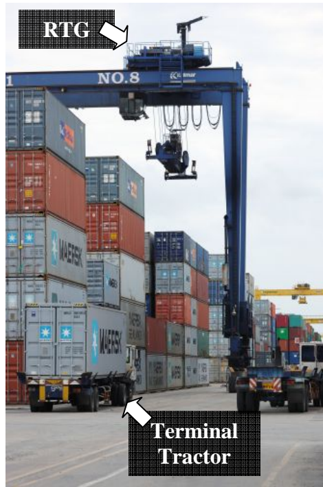
Figure 3. Rubber Tired Gantry Crane and Terminal Tractor: A terminal tractor in the buffer area waiting on a RTG. The RTG will move the containers from the terminal tractor to place the container in the block (From Container Shipping Information Service, 2008).
