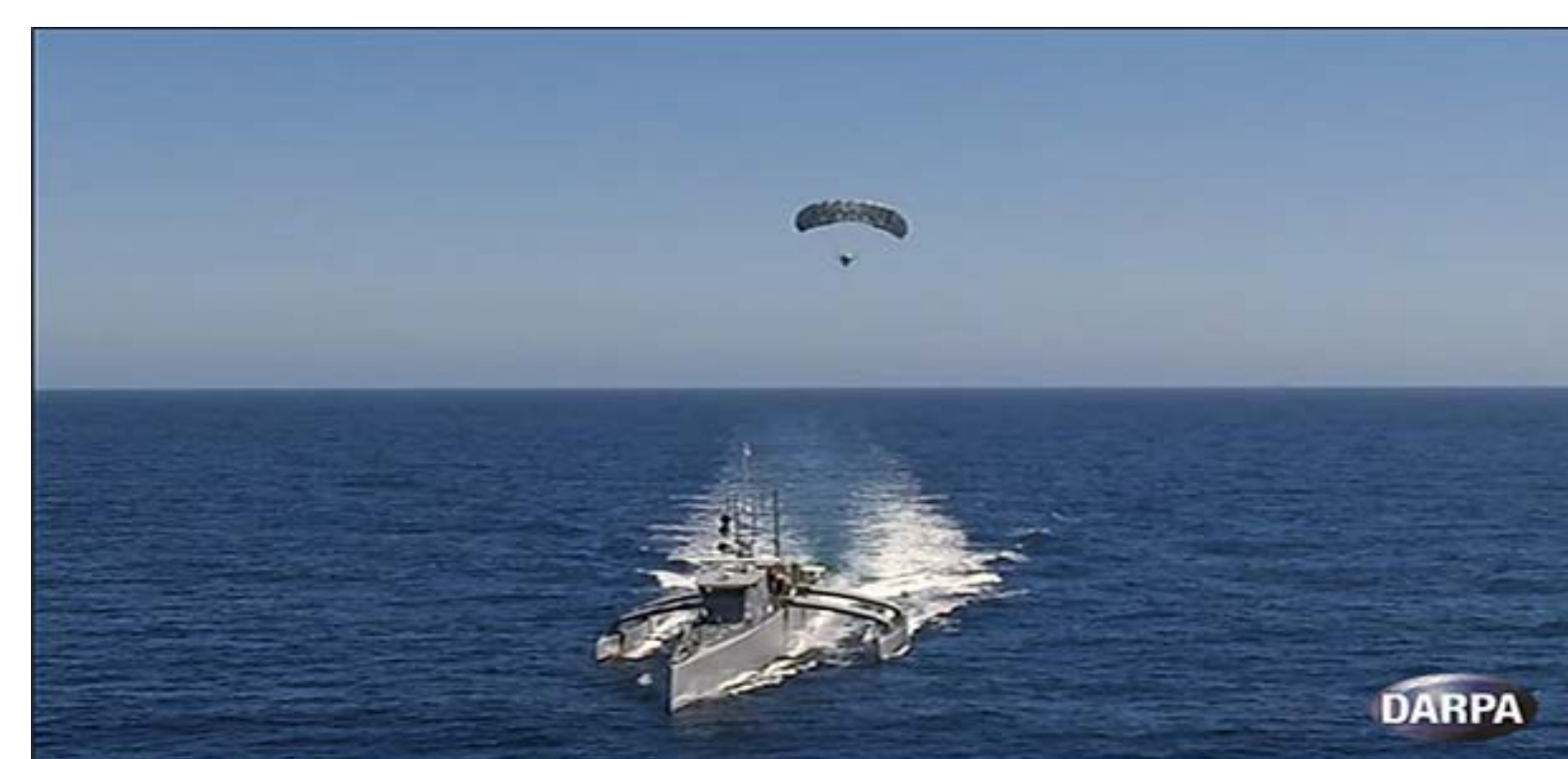
MDUSV with the TALONS deployed. A potentially important communications link for MCM missions
