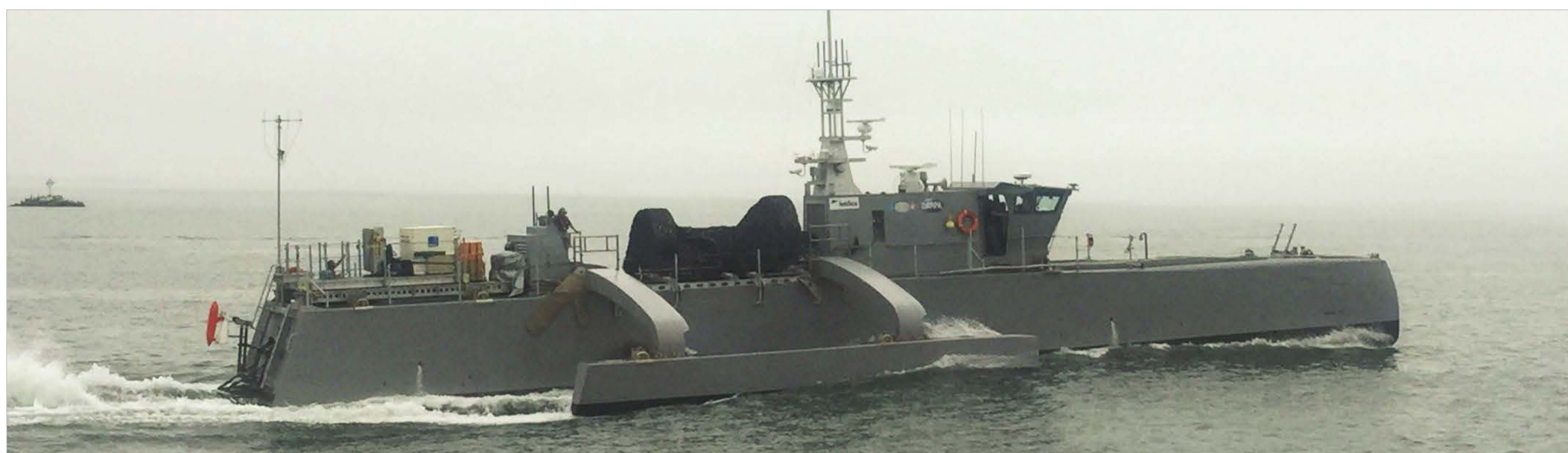
MDUSV Testing a High Temperature Superconducting (HTS) MCM System
