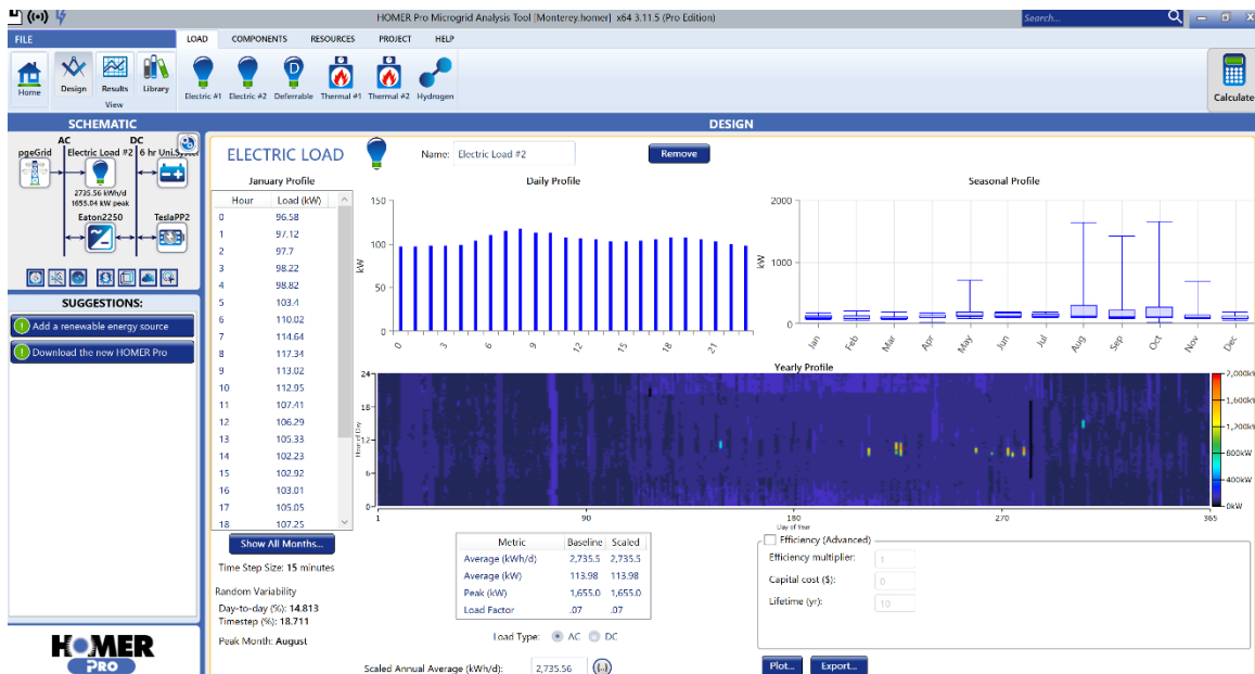
Figure 21. HOMER Electric Load Interface
