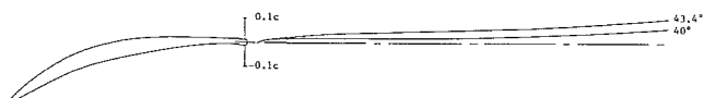
Fig. 9 Location of the wake minimum velocity from LDV and calibrated pressure probe measurements
