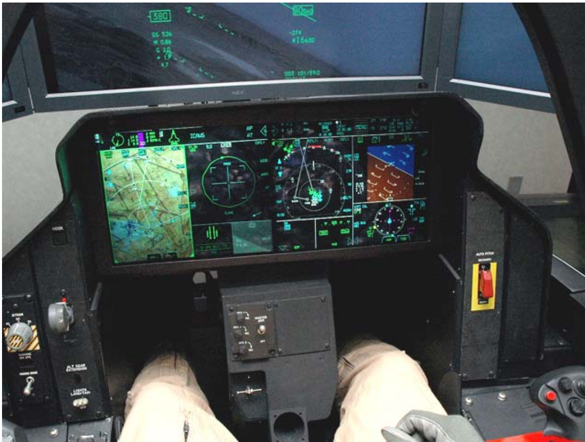
Figure 4. JSF cockpit with LCD display suite (From: briefing received from PVI Team at Lockheed Martin, Fort Worth, TX)
