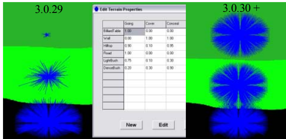
Figure 3. Line of sight determination in version for this study versus subsequent versions. We see the desirable LOS characteristics of version 3.0.29 on the left, versus subsequent versions on the right. [Best viewed in color]
