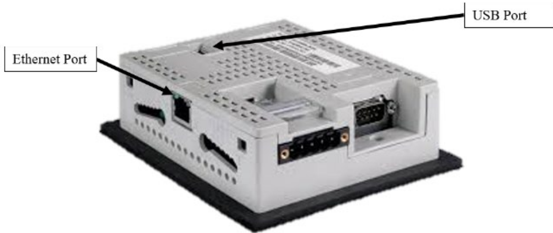
Figure 25. PanelView 800 Graphics Terminal rear view. Source: [27].
