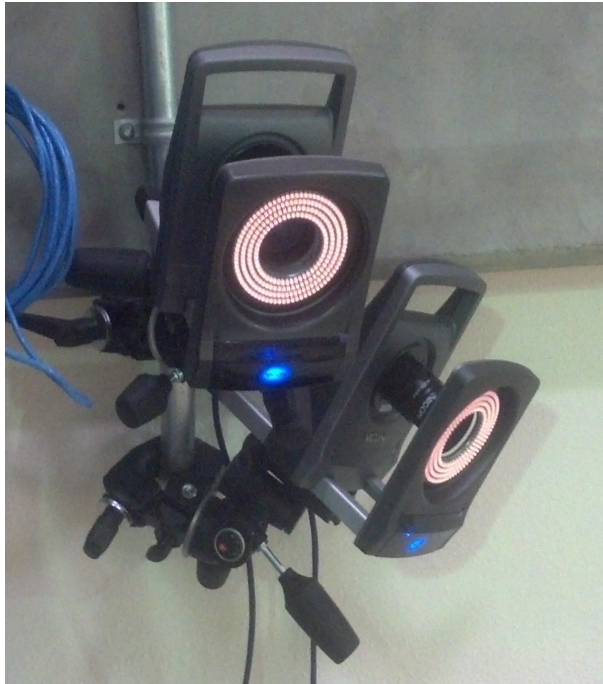
Figure 4.2: Two of the ten Vicon motion capture cameras used to capture true position and orientation of the AR Drones used in this project.
