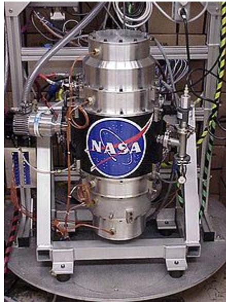
Figure 21. The NASA G2 experimental flywheel: capable of speeds up to 60,000 RPM. From [12]
