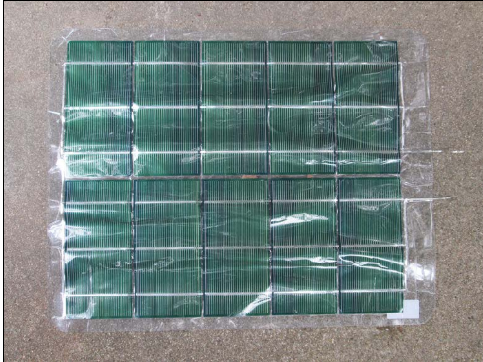
Figure 12. Constructed CIGS solar cell array.
