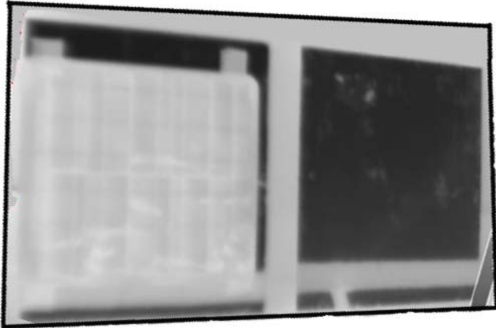
Figure 32. Comparison of aluminum plate with a solar array (left) to a bare aluminum plate (right) using a “white hot” setting.
