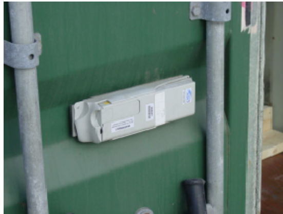
Figure 17. RFID Tag used during OIF3 to track containerized cargo (Courtesy of Henry Cook)
