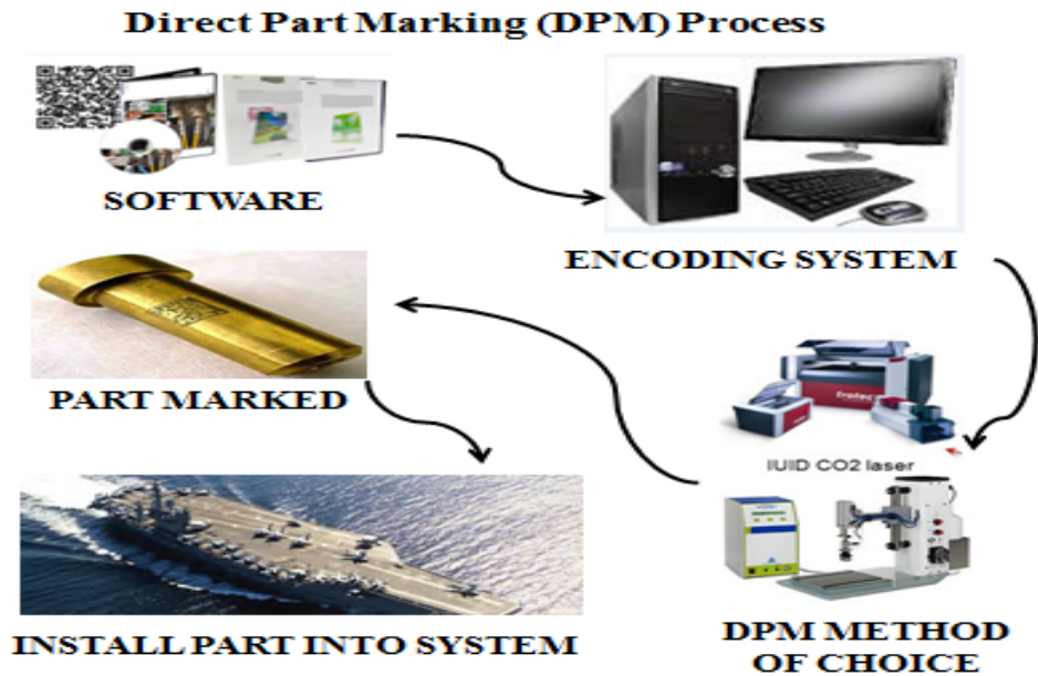
Figure 16. DPM Process (after UID Forum, 2010).
