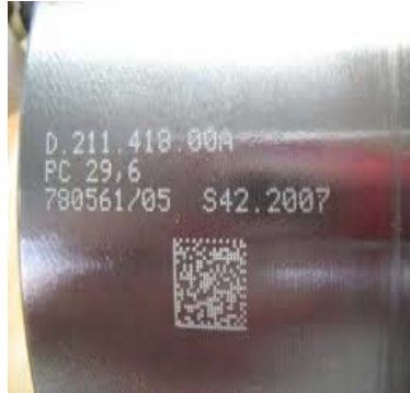
Figure 19. Laser Etching (from SIC Marking, 2014).
