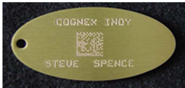
Figure 17. Dot Peening Example (from Spence, 2005).
