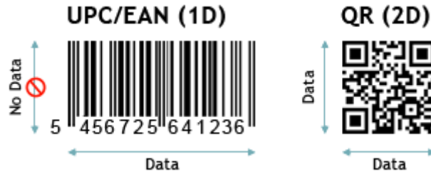
Figure 5. 1D vs. 2D Barcodes (from Schottmuller, 2011).
