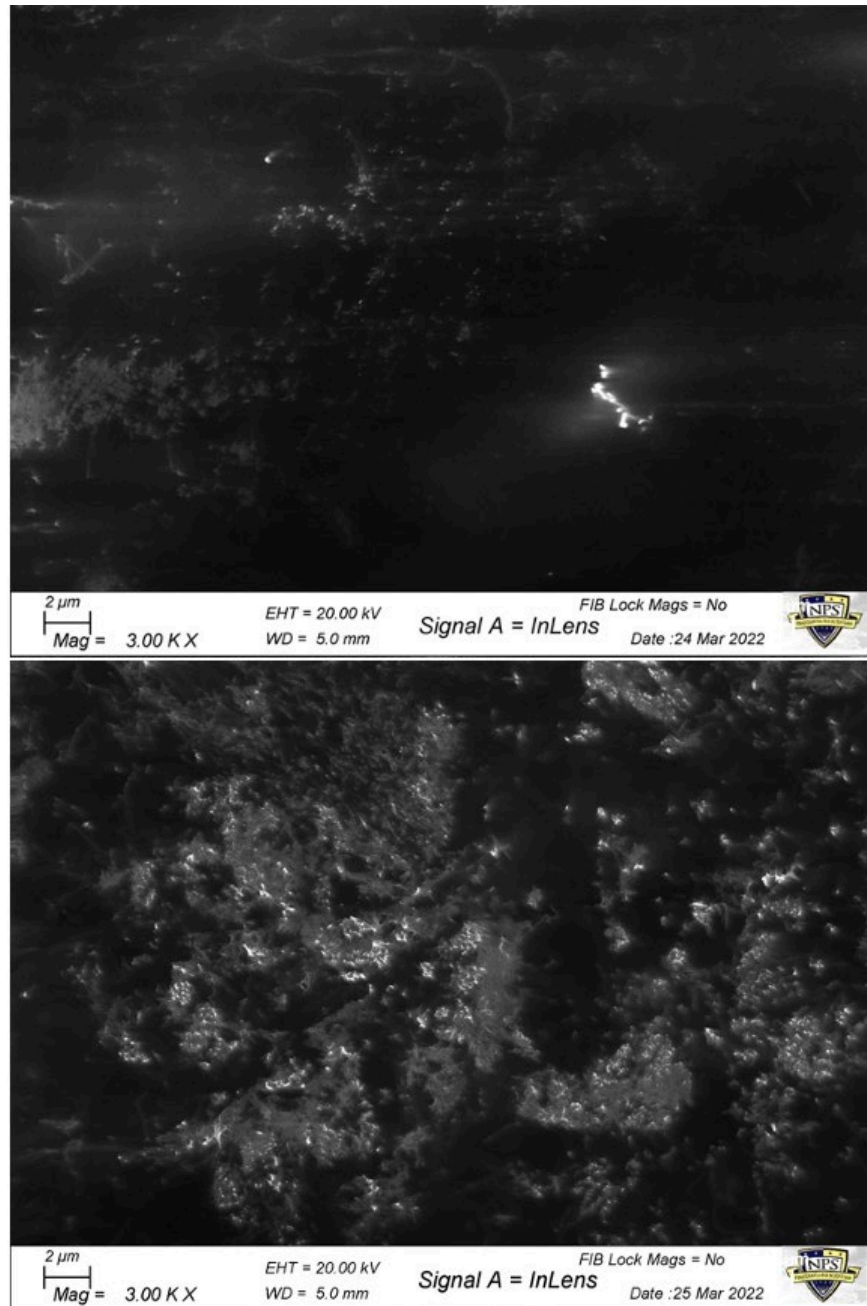
Figure 24. Top: 1 wt% BNNB 0.5 wt% CNT SEM image 3000x, Bottom: 5 wt% BNNB 0.5 wt% CNT SEM image 3000x
