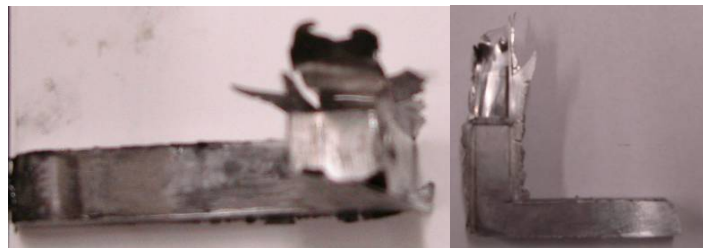
Figure 9 First pressed billet showing significant side- and back-extrusion
