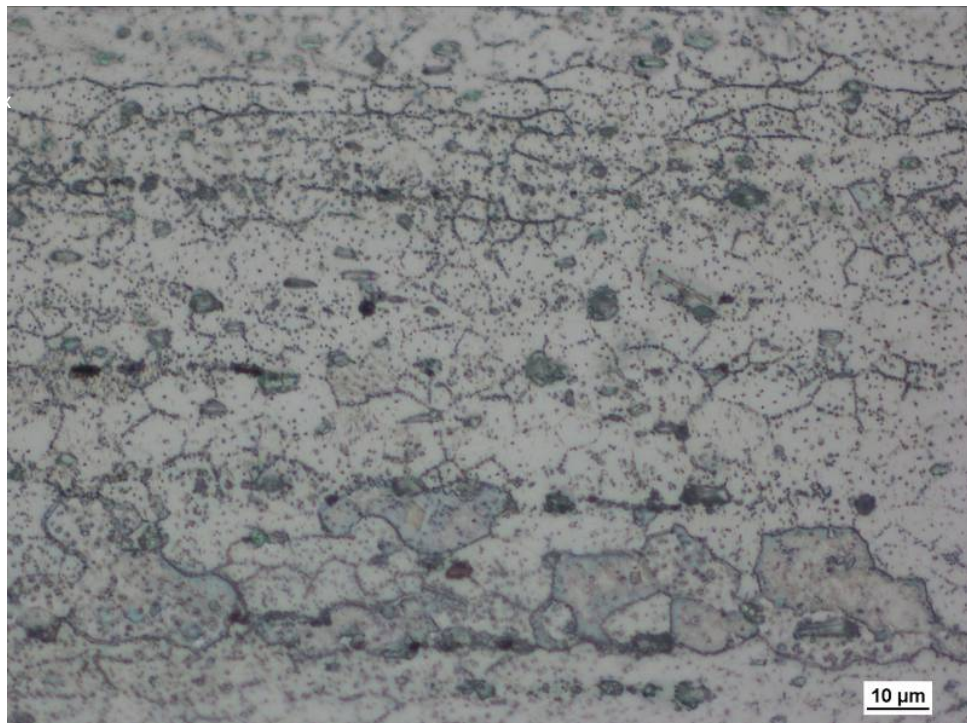
Figure 29 Highest magnification of AA6061-O along the flow plane
