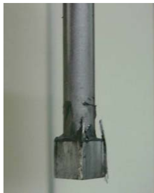
Figure 15 Evidence of back-extrusion on the plunger
