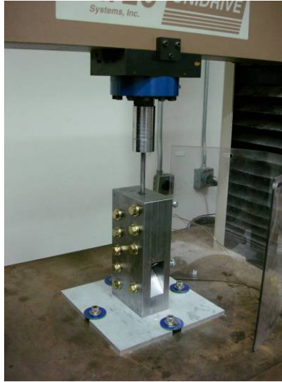
Figure 14 Photograph of new ECAP assembly on Satec pressing machine
