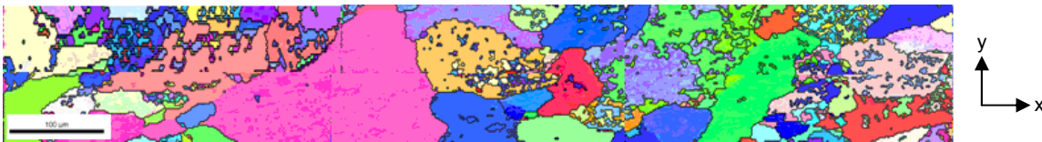
Figure 22 Representative OIM image of annealed, unpressed AA1050 flow plane/top plane
