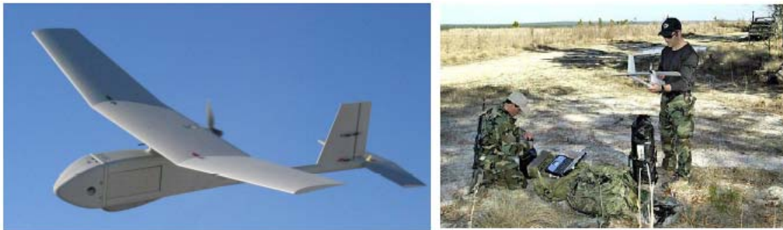
Figure 8. Raven B (left), An Operator and Observer Team Assembling the SUAS (right). (From: Lifschitz et al., 2007)
