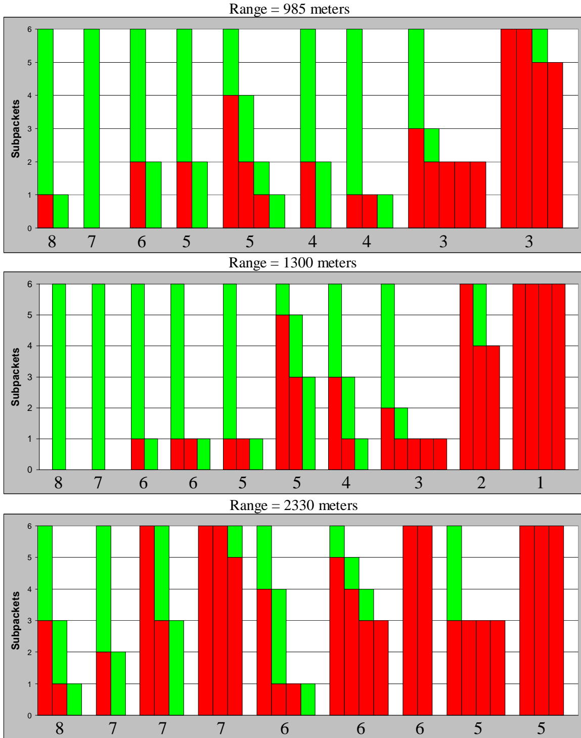
Figure 8. Transmission results for all three test geometries. A dialogue is represented as a group of bars, with power level noted below each. As explained in Figure 2, one bar represents a single transmission. The total height of the bar represents the total subpackets sent in that transmission; the height of the red portion of a bar represents those subpackets that were received corrupt. If the last bar (transmission) of a dialogue is fully green, the file was successfully sent.
