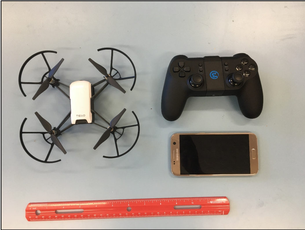
Figure 8. Ryze Tello Drone with DJI Avionics Next to Controller and Phone
