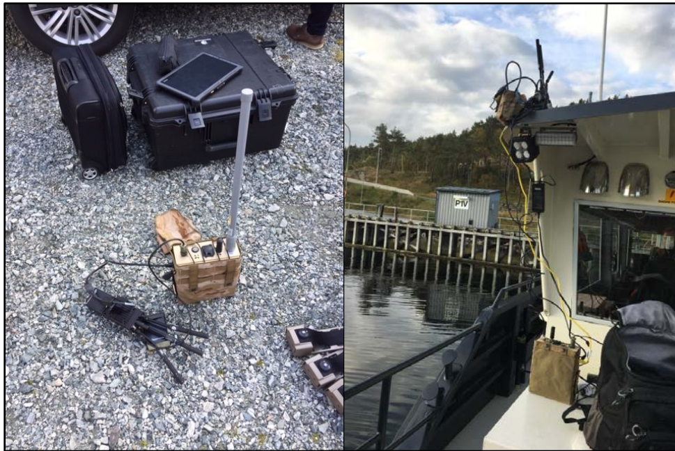
Figure 5. SkyView RF Sensor in Dismounted and Vessel Mounted Configurations
