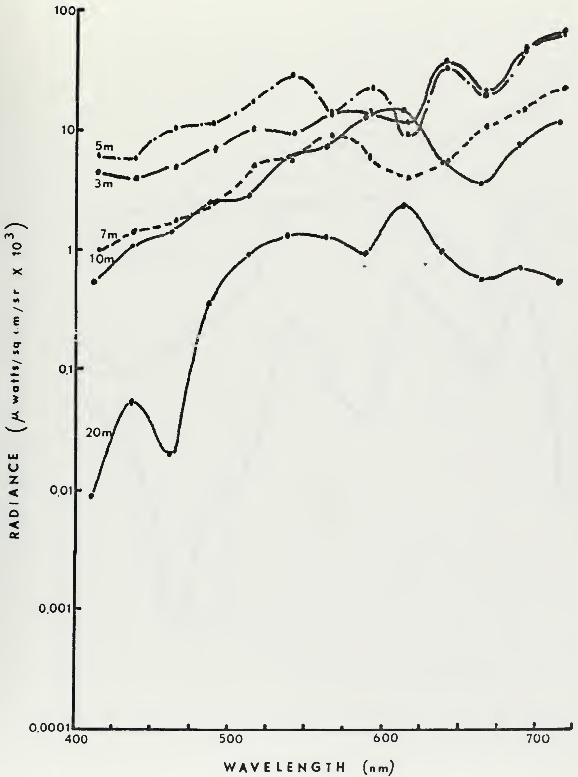
FIGURE 24. SPECTRAL RADIANCE DISTRIBUTION WITH DEPTH AT \theta = 90^\circ AND \phi = 0^\circ , STA 1
